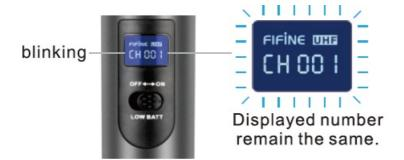
3. Turn the receiver on while the screen is flashing. The receiver indicator will flash green and red alternately and then turn green again.
