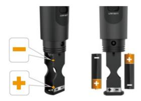
• Insert 2 AAA batteries to the receiver. Make sure the battery polarity is correct installation and the door is closed completely.
