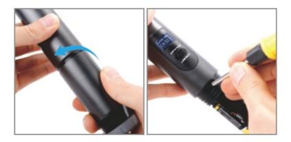
3. The Led screen is blinking if you do it right.(Note: The figures on Led display will not change) Note: The receiver must remain OFF at this moment.
