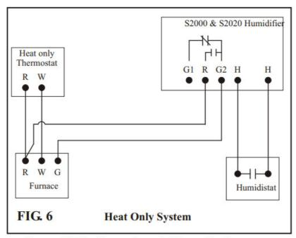
Connect field wiring as shown in Figures 5 or 6.
