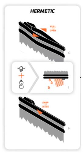
Release the HERMETIC closure and snap it shut (Fig. H).
