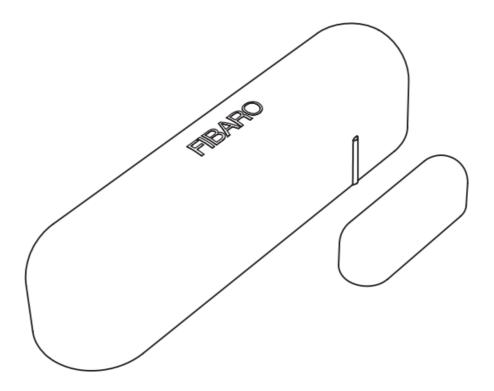
**FIBARO Door/Window Sensor** is a HomeKit-enabled Hall effect sensor using Bluetooth® low energy wireless technology. Along with detecting opening and closing, the accessory measures the ambient temperature. Opening is detected by separating the sensor's body and the magnet. Tampering is detected whenever the accessory is detached from the surface or casing is opened.
