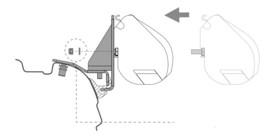
• Before tightening the screws, make sure that the awning position doesn't prevent the opening of the rear door.
