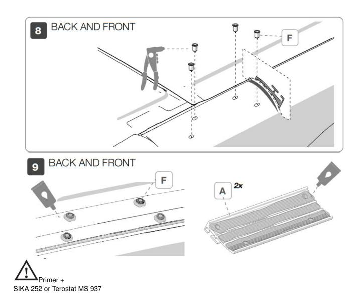
Important: use of SIKA 252 (or Terostat MS 937) adhesive is essential for fi xing the bracket (brackets).
