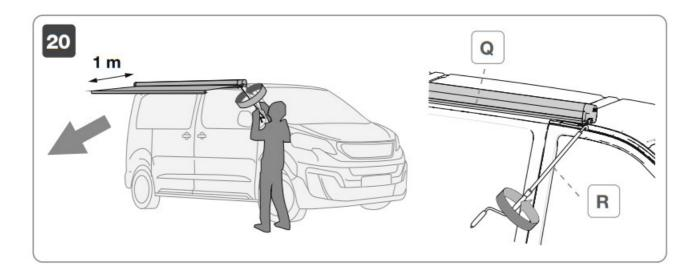
In order to avoid unnecessary strain on the awning as well as on the vehicle side, we suggest to take out the legs at about 1 m from the opening.
