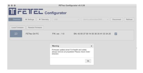
choose USB and select the correct COM Port and press connect. You should see the FETtec FC G4 as shown. Click "Remote Firmware" button and select the latest available firmware. Press "Flash selected!" FC is flashed now! Settings can be made in the KISS GUI.
