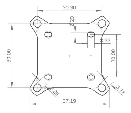
Maximum outside dimensions:  $37.2 \times 37.2$ mm, without outside tips  $30 \times 30$ mm **Mounting hole arrangement:**
