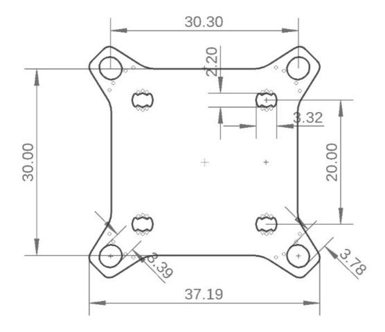
Maximum outside dimensions: 37,2 x 37,2mm, without outside tips 30 x 30mm Mounting hole arrangement:
