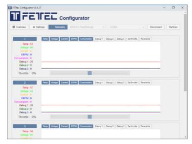
In the Telemetry page you can spin the motors, view and debug the motor telemetry.
