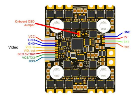
The 8 pin connector combines all necessary connections for analog or digital VTX and camera. It includes:
