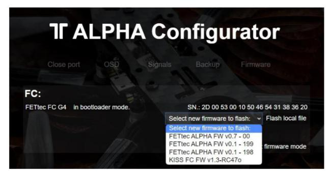
6. Confirm to flash FETtec ALPHA firmware by pressing "OK"
