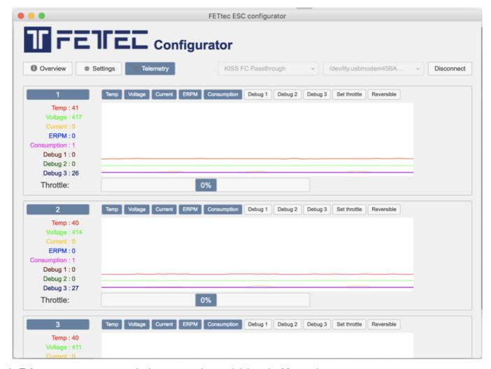
In **Telemetry** page you can spin the motors, view and debug the Motor telemetry.
