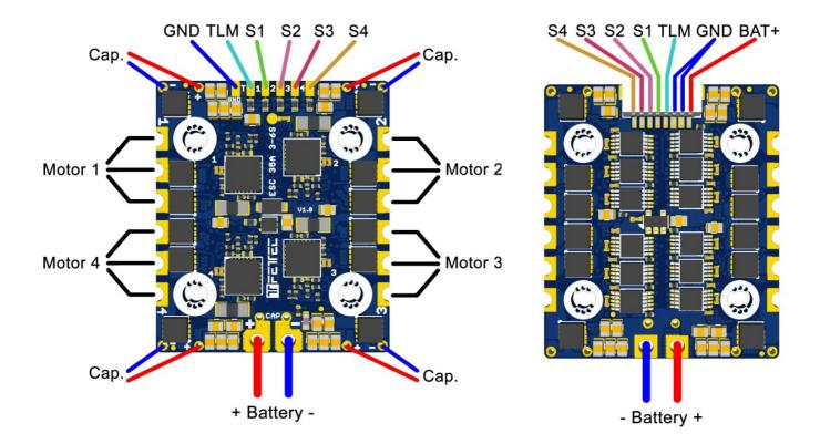
S1 – S4 – Motor Signal 1-4 TLM – Telemetry (Serial) GND – Reference Signal Ground
