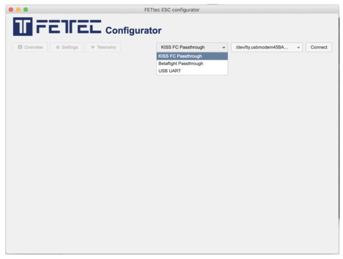
Mainpage to connect to the ESC. Please select correct connectivity type and serial/COM port.
