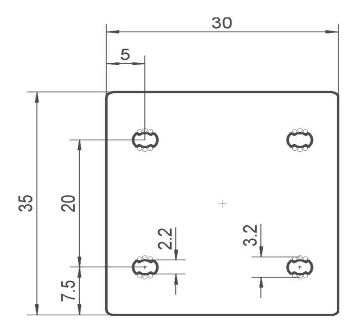
The FETtec 4in1 ESC 35A comes with a 20 mm x 20mm mounting hole layout designed for M2 and M3 screws. Original is for M2 while you can use a screw driver and force it into M3 by rotating it inside the hole carefully. Do not file the mounting holes as this may cause damage.
