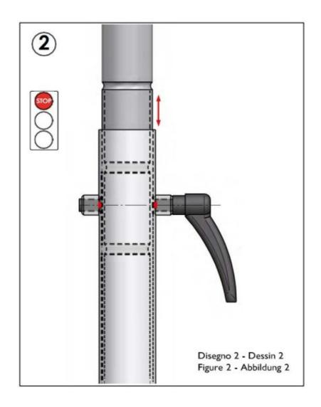
THE NOTCH POSITIONING FOR HEIGHT ADJUSTMENT IS: WRONG.
