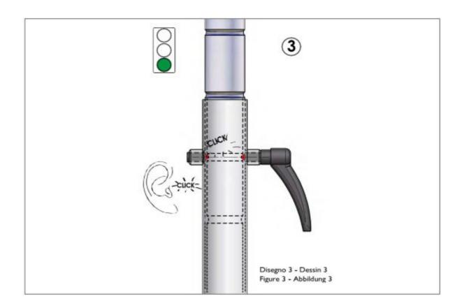
THE NOTCH POSITIONING FOR HEIGHT ADJUSTMENT IS: CORRECT.
