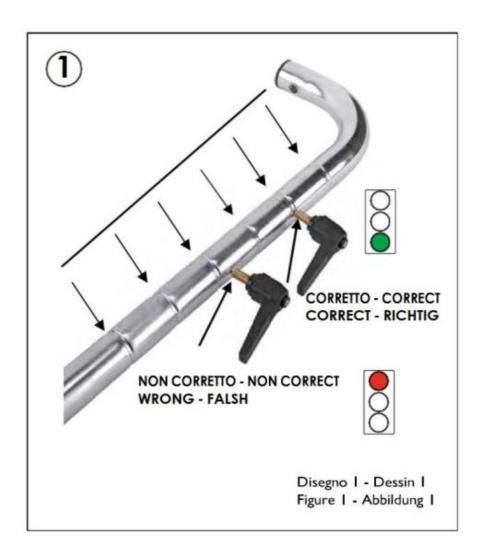
THE HEIGHT OF THE PARALLEL BARS IS CORRECTLY AND SECURELY ADJUSTED, ONCE THE FASTENER TIGHTLY SITS IN ONE OF THE SPECIFICALLY DESIGNED NOTCHES
