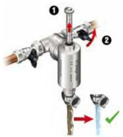
5. Close the inlet valve. Close the drain valve.
