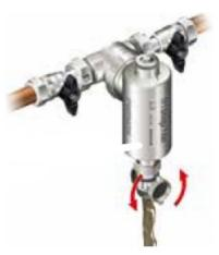
4. Remove the magnet. Slowly open the inlet valve to control the flow. Flush out the filter until the water runs clear.
