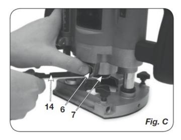
Only use cutters with a shaft diameter which corresponds with the size of the collet. Only use cutters which are suited for the maximum speed of the machine. The cutter diameter should not exceed the maximum diameter (see 'Technical specifications'). Never tighten the collet nut, if there is no router bit in the collet; the collet may be damaged.
