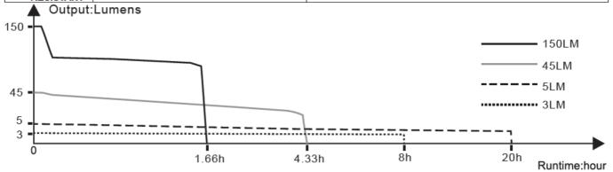
**Note:** According to the ANSI/PLATO FL1 standard, the above specifications are from the results produced by Fenix through its laboratory testing using the built-in 275mAh Li-polymer battery, under the temperature of  $21\pm3^{\circ}$ C and humidity of 50% - 80%. The true performance of this product may vary according to different working environments.
