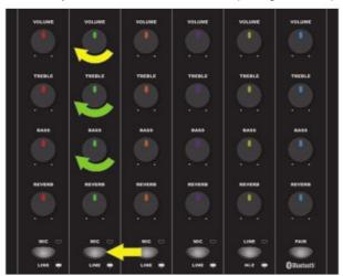
10. **SETTING TONE/REVERB**: Starting with each TONE control (TREBLE, BASS) in the center-detented position (flat equalization), set each TONE control to preference for best clear and consistent sound coverage throughout the area. REVERB controls (green arrows) are not center detented; set these to preference:
