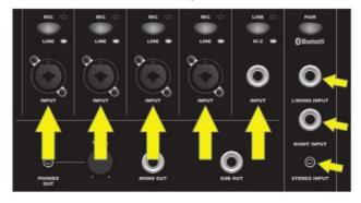
6. **INITIAL VOLUME/REVERB**: Turn MASTER VOLUME knob, all channel VOLUME knobs and all REVERB knobs fully counterclockwise to start:
