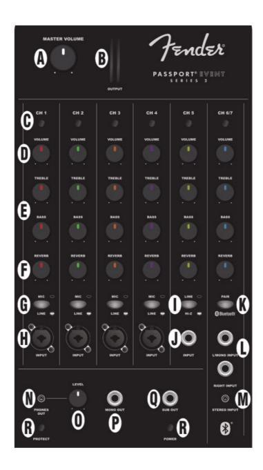
A. MASTER VOLUME: Adjusts overall loudness. No sound is produced at full counterclockwise position.
