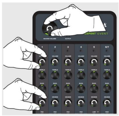
7. Turn on all equipment connected to the Passport first, then switch the Passport on. The Power LED on the Passport should illuminate green (Protect LED will illuminate briefly).
