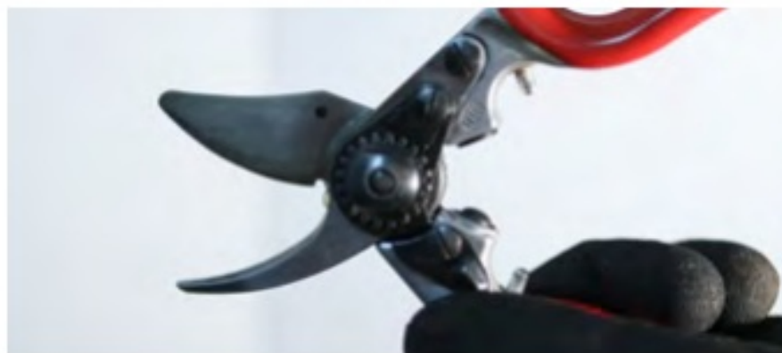
6. Blade crossing should be between 1/2 & 2/3 .
