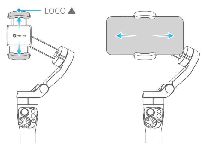
Keep the logo of the smartphone holder upward. Keep the smartphone holder in the center. If the smartphone is tilted, please move the smartphone left or right to make it horizontal.
