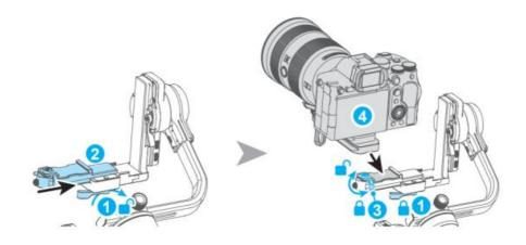
It is recommended to push the camera against the tilt axis. Unlock ② to move the camera left or right according to camera's width to adjust, then lock ③.
