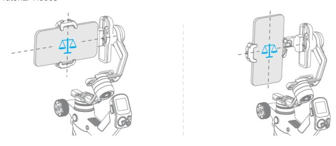
Place the smartphone in a roughly balanced position.
