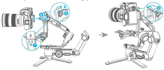
**Remove:** Please refer to the remove steps for horizontal mounting. Unlock the quick release plate safety lock  $\P$  , remove the quick release plate while pressing anti-drop column  $\P$ .
