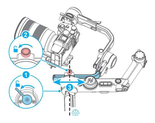
The pan axis is balanced when the camera can stay still and horizontal to the ground.
