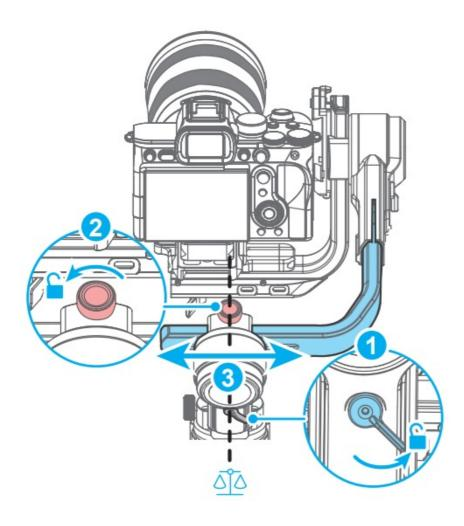
The roll axis is balanced when the camera can stay still and horizontal to the ground.
