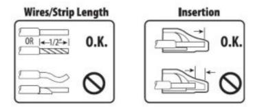
NOTE: If the jacket of the cable is not in the U wago connector, ensure the strip length is correct and/or verify the wire is fully inserted.
