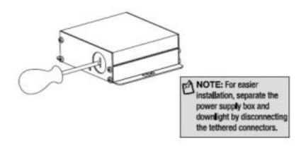
4. Open the power supply box cover. Feed the supply wire into the knockout hole using a 3/8 in. clamp connector (not included) and make all the connections inside the power supply box using wago connectors. Connect the 120V line (black) wire to the black wire. Connect the neutral (white) wire to the white wire. Connect the ground (green) wire to the green wire. This power supply box needs to be grounded.
