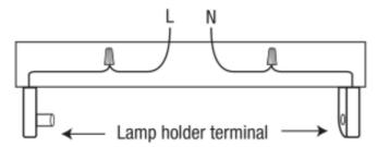
**NOTE:** Installers should not disconnect existing wires from lamp holder terminals to make new connections at lamp holder terminals. instead installers should cut existing lamp holder leads away from the lamp holder and make new electrical connections to lamp holder lead wires by employing applicable connectors.
