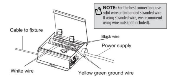
**5** After inserting the supply wire into the wago connectors, double-check the connection by following these simple tests:
