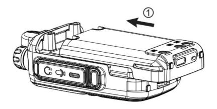
To remove the battery pack, pull downward the battery latch in the middle of the transceiver, then slide downward the battery away from the transceiver's body, and lift the battery from the transceiver's body.
