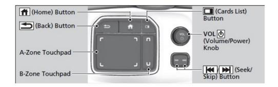
VOL (Volume/Power) Knob: Push to turn the audio system on and off. Turn to adjust the volume when the audio system is on. / (Seek/Skip) Button: Press to change the station, channel, song or file.
