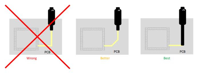
Figure 8-3-2: Recommended Trace Connects Antenna and the Module
