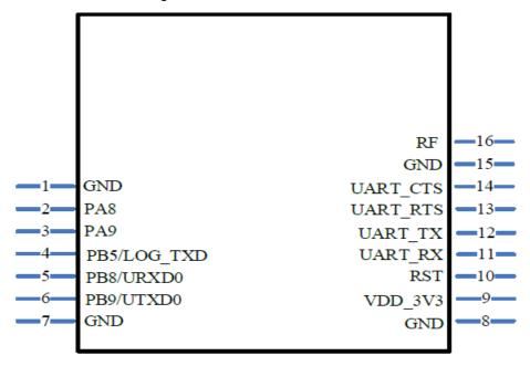
Figure 3-1-2: FSC-BT9104DI PIN Diagram (Top View)
