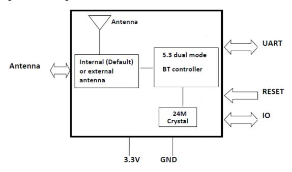
Figure 3-1-1: FSC-BT9104DI Block Diagram
