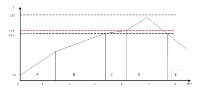
Figure 6-1 Typical Lead-free Re-flow
