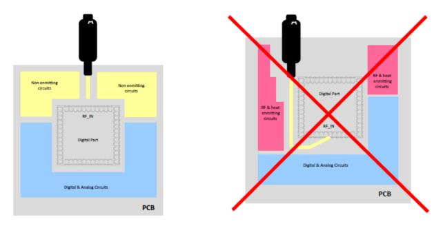
Figure 8-3: Placement the Module on a System Board
