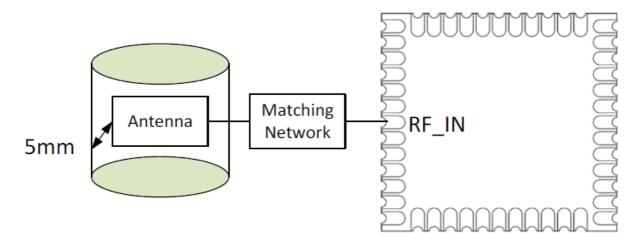
Figure 8-3-1: Leave 5mm Clearance Space from the Antenna
