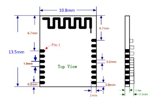
Figure 7-1 FSC-BT9104DI footprint Layout Guide (Top View)
