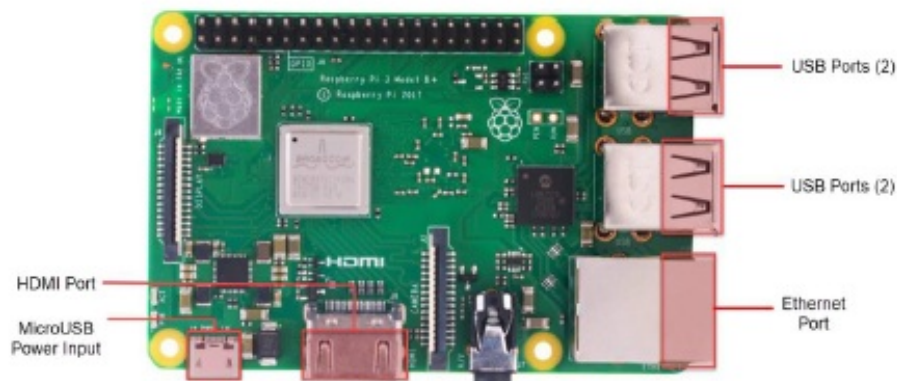
Figure 7. Raspberry Pi Model 3B+ Connections
