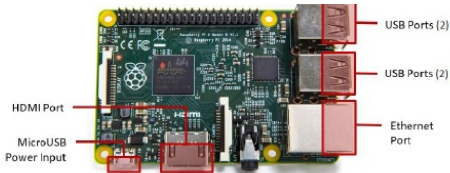
Figure 5. Raspberry Pi 2 Model B Connections
