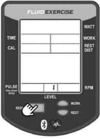
**STEP 3** Turn the handle to Level 2. Press Reset. The display will now show Level 3.
