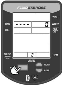
**STEP 4** Repeat for 3,4,5,6,7,8,9,10. Level 10 Press Reset. Repeat the steps back to level 1. Calibration is complete.
