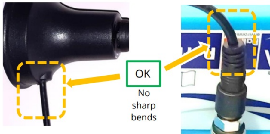
Figure 23. Protect from sharp bends (especially near connectors)
