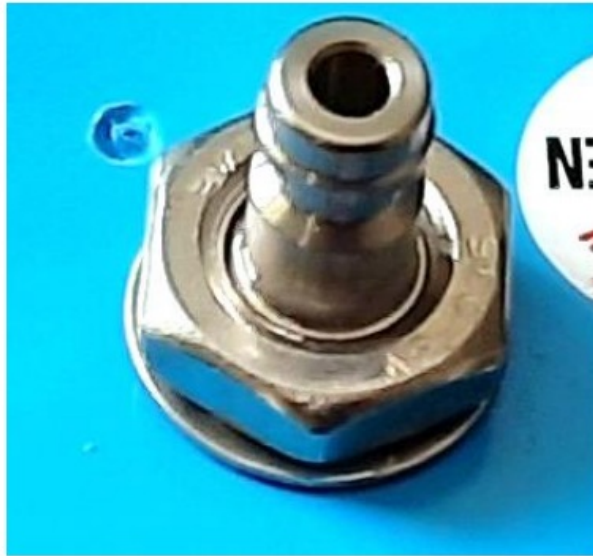
Figure 10. Connection to an internal water pressure transducer
