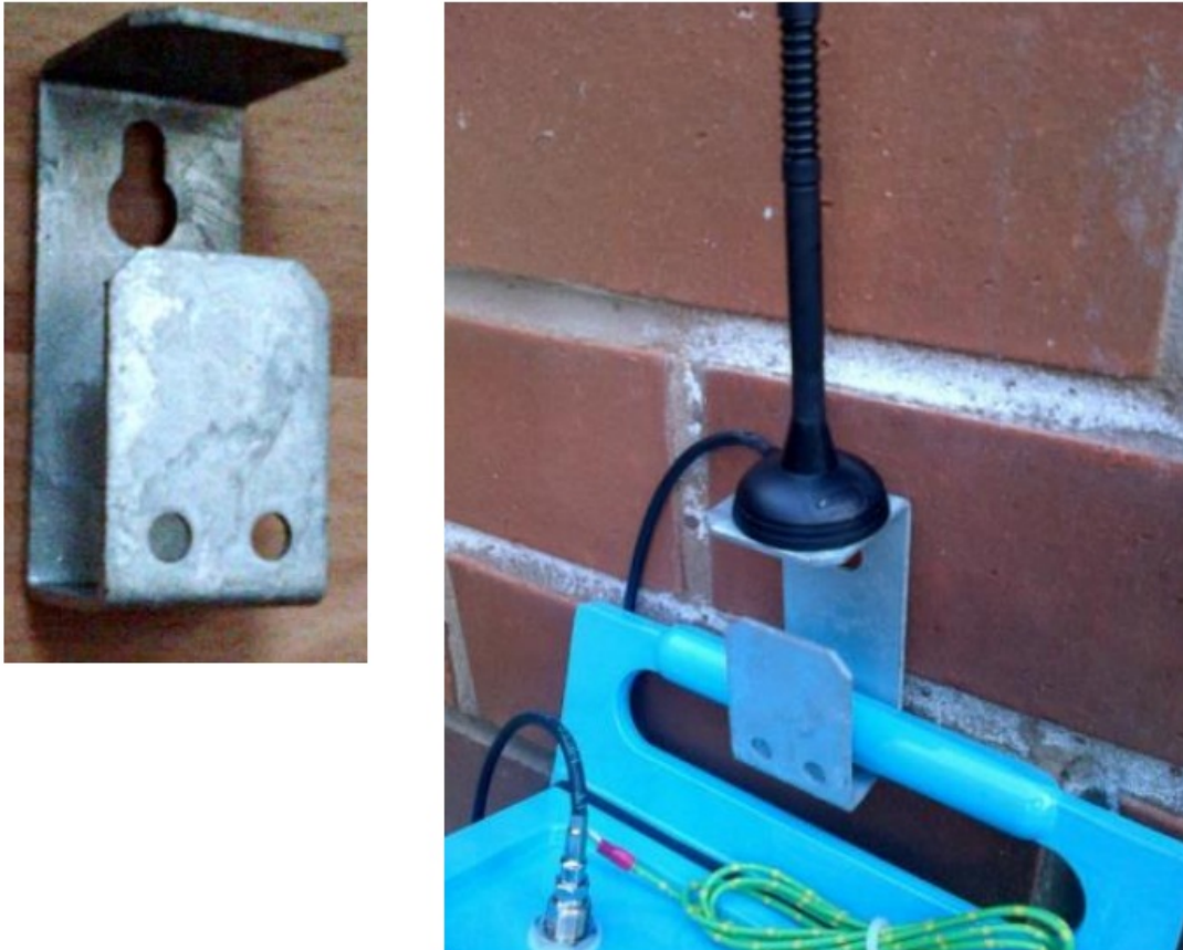
Figure 11. Example installation of Multilog2 using a suitable wall-mount bracket.
