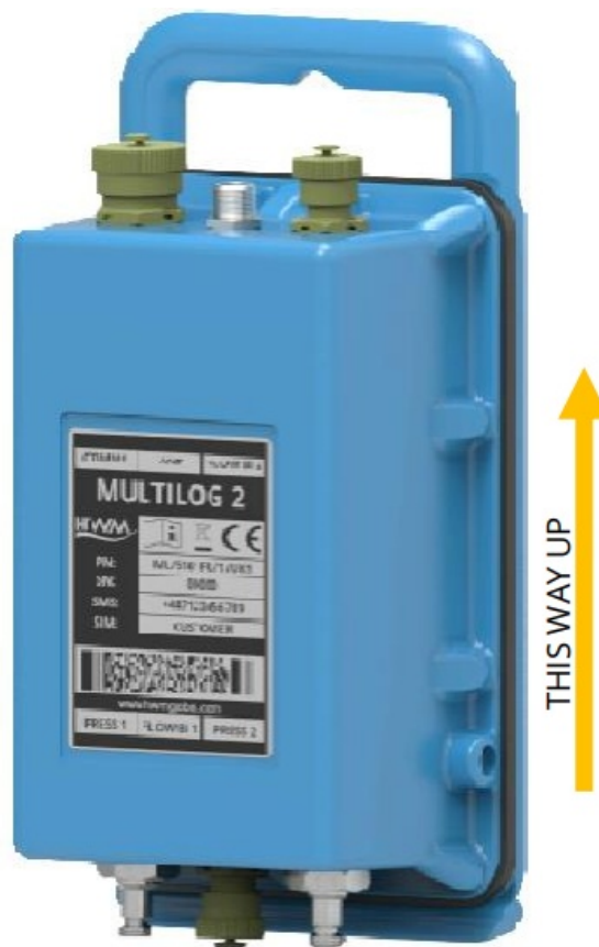
Figure 1. An example Multilog2 Logger. Shows correct orientation for best battery life.
