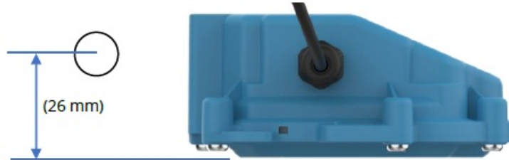
Figure 7. Offset (typical) of RadarSens from center of bracket arm (round)
