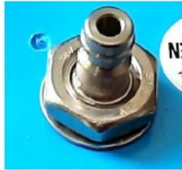
Figure 11. Connection to internal water pressure transducer
