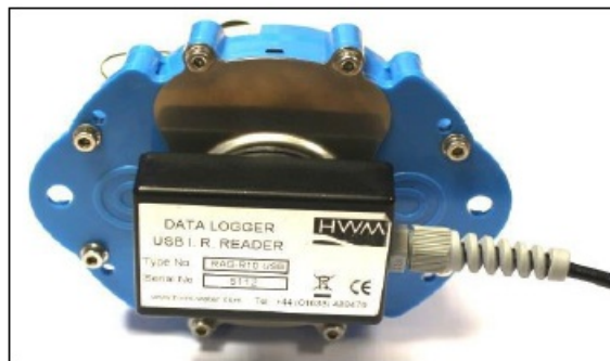
Figure 6. IR Reader coupled to the logger for communications.
