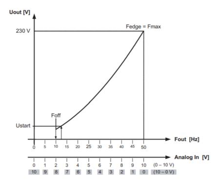
Analog In Speed setting signal 0 - 10 V / 10 - 0 V
