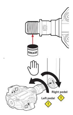
3. Screw with torque 35Nm ± 5Nm
