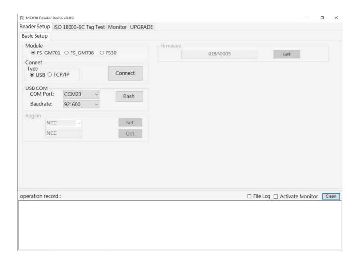
Please select USB as Connection, Choose the corresponding Serial Port and Baud Rate (default baud rate is 921600). As illustrated below:
