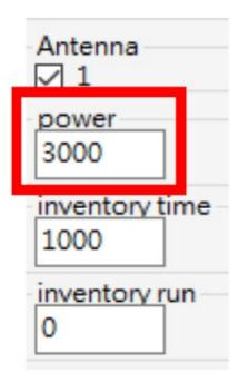
The output power range is 0 – 33dBm. Default RF output power is 30dBm.
