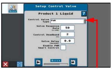
• If using ACE PWM pump, change the coil frequency to 122.
