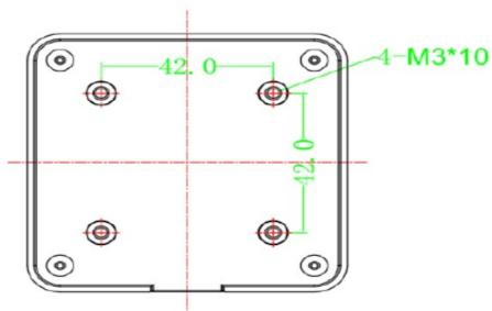
The above image is an upward view of the device, using four M3×10 self-tapping screws.
