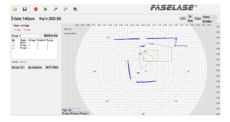
As shown in the figure above, "current input group 4" means that the connected level status of IO\_In1 and IO\_IN2 of this Lidar is low, in the wiring state of IO\_In, the Lidar calls protected area 3 in current input group 4. In this case that the I/O input is not connected to any external circuit, the default current input is group 4.
