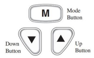
The instrument has three push buttons; "Up," "Down," and "Mode" buttons; that control the modes of operation. The "Mode" button is used to change the function of the LCD display and to access submenus and adjustable settings. The "Down" and "Up" buttons are used to modify the settings.
