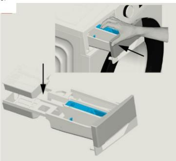
Replace with a new filter and reinsert the drawer
