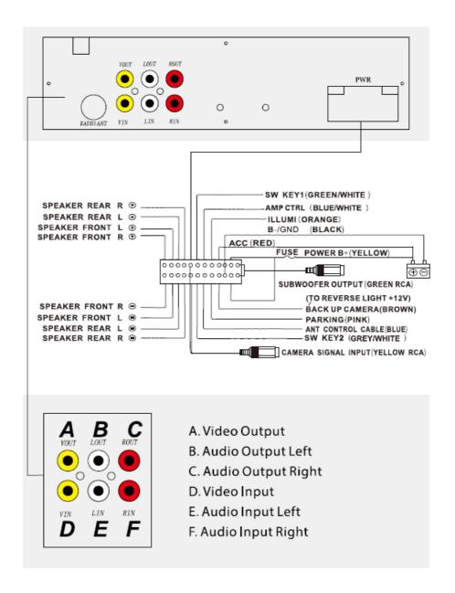
Wiring - Color Wiring
