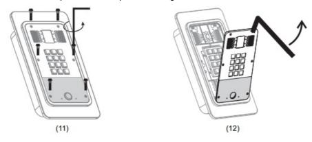
• B.With Phillips screwdriver, unpack Iha frame panel and Iha main part of intercom as diagram
