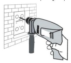
2. The white rubber plugged into the wall and the flush-mounted bracket fixed with screws to the wall, and insert the flush-mounted bracket cover plate stuck on the flush-mounted bracket.
