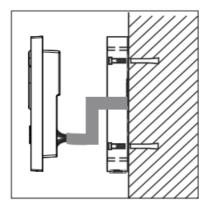
5. Power on the device, If it works normally, then use the screws to fix A12 to the wall-mounted bracket, and the installation is complete.
