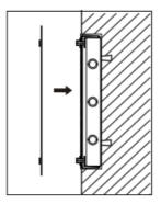
3. Fix the sealing silicone ring on the back of A12 according to the hole position.
