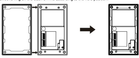
4. After connecting the power cables, network cables, and security interface cables, place the A12 on the flush-mounted bracket.
