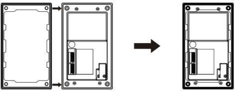
4. After connecting the power cables, network cables, and security interface cables, place the A 12 on the wall-mounted bracket.
