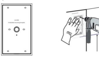
2. The white rubber was plugged into the wall and the wall-mounted bracket fixed with screws to the wall.
