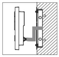
5. Power on the device, If it works normally, then use the screws to fix A 12 to the flushl-mounted bracket, and the installation is complete.
