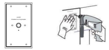
2. The white rubber plugged into the wall and the wall-mounted bracket fixed with screws to the wall.
