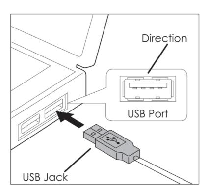
It's plug and play. Connect the keyboard to computer by inserting USB jack to your computer USB port
