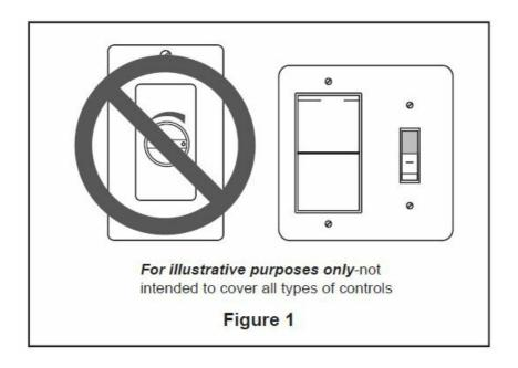
1. **IMPORTANT:** Using a full range dimmer switch (not included) to control fan speed will damage the fan. To reduce the risk of fire or electrical shock, do not use a full range dimmer switch to control the fan speed. (Figure 1)
