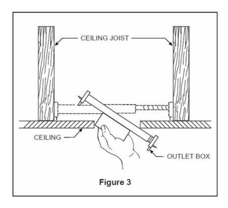
Paired with a deep box, this hanger is meant to span between two joists and takes the place of wooden blocking.
