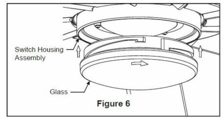
6. Secure the glass to switch housing assembly by twisting in a clockwise direction. Twist the glass gradually until it snaps onto the switch housing assembly. Do not over-tighten. (Figure 6)
