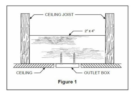
• A 1/2-in.-deep pancake box is meant to be screwed to a joist or block. It's used if only one cable is coming into the box. It is also available in a saddle-mount configuration.
