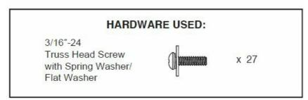
1. Position blade over the hub of motor assembly with the threaded posts showing. Make sure the bottom edge of the blade is fully seated against the hub of motor assembly and tighten 3/16"-24 truss head screw with spring washer/flat washer. (Figure 1)
