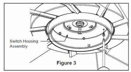
3. Remove one of the three screws in the switch housing assembly. Retain the screw for later and slightly loosen the remaining two screws. (Figure 3)
