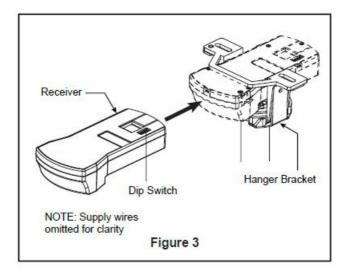
2. Slide the receiver into the hanger bracket before wiring as shown in figure 3.
