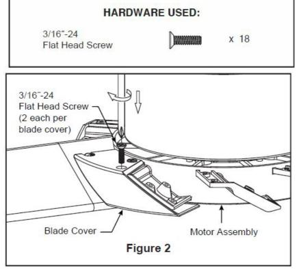
2. Secure the blade cover to the hub of motor assembly using 3/16"-24 flat head screw. (Figure 2)
