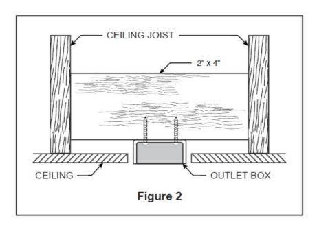
• A 2-1/4-in.-deep box can be attached to blocking between joists and is roomy enough to handle more than one cable.
