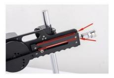
5. Install accessories and connect the connector Install into the socket. (All attachment installation methods are the same)
