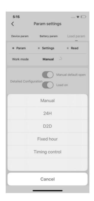
Step 4: Load mode – manual mode. 'Manual default ON', when the device is turned on, the load is open. 'Manual default OFF', when the device is turned on, the load is close. The second soft key can open the load manually (by clicking on it).
