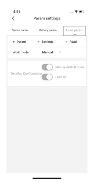
Step 2: Click 'work mode' to select the working mode (the option is determined by the actual device).
