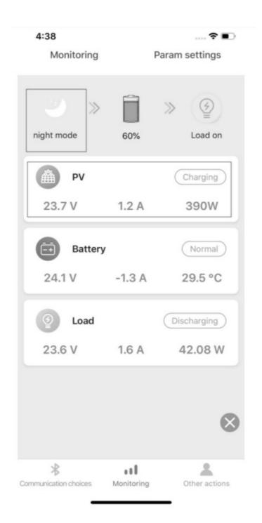
Step 2: Click 'PV', to access the page of PV details. On this page you can read PV voltage, PV current, PV power, charging energy today, total charging energy as well as energy generated graphs of 60 days.
