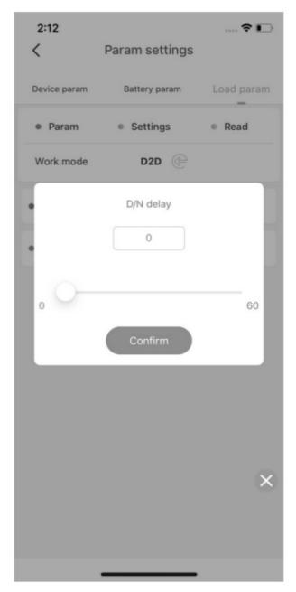
Step 7: Work Mode – Fixed lighting hours. The light on time, Day/Night Threshold voltage and Day/Night delay time can be set.
