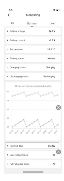
Step 3: Should there be problems with indications on PV, battery or load, an alarm message will be presented red color on 'Battery status'
