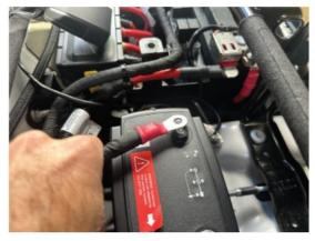
• The CTEK Smartpass has 3 cables connected to it that need to be disconnected and removed. The first is the 4 gauge red cable connected to the Left side (A) stud. Disconnect on the CTEK.
