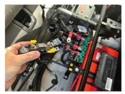
• The other side of the CTEK Smartpass (Right side terminal with a battery icon) has a small positive cable that runs to a fuse holder on the passenger side (Pictured). You will remove this cable, the fuse holder and the other positive cable running to the AUX battery. (Second cable not pictured but it is the cable running from this fuse block to the AUX battery.)
