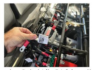
Removal of CTEK Smartpass and mounting bracket: Now that all of your cables are removed, use a 10mm Socket wrench to remove the 4 M6 screws holding the CTEK to the body of your vehicle.
