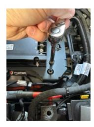
• The M6 Flanged Screws go in the 4 locations indicated by the yellow arrows in the picture above. Use a 10mm socket wrench to install. YOu may need a a ujoint socket adapter ont the two screw locations that are on an angle.
