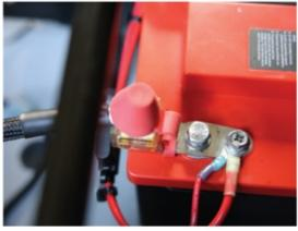
• The Wire that runs to the AUX battery positive side will use the provide EATON fuse holder and one of the 60a fuses provided. This fuse holder has a 3/8 hole so it can be mounted to a screw down positive terminal (pictured on the Redarc Battery) or it can be used on a standard stud terminal mount for the AUX battery (Terminal mount not provided).
