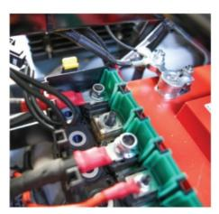
• The Wire that runs to the truck battery positive bussbar (in front on the AUX battery, will need to have a new fuse placed in the location where the 300a fuse was removed. Take ove of the provide 60a fuses and secure the terminal in the location pictured.
