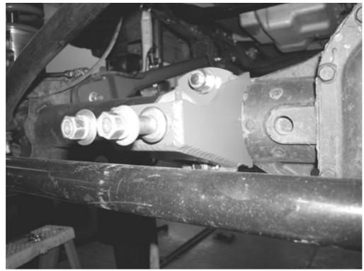
4. Working from the driver side of the truck, locate FT 30149 tie rod end bracket and position it 2" from the outer tie rod end. Using the Supplied FT740U U-Bolt and 3/8" hardware attach the bracket to the tie rod end. Leave loose at this time. SEE PHOTO BELOW.
